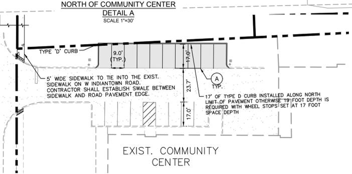
CONSTRUCTION AND MATERIALS SHALL BE IN ACCORDANCE WITH THE TOWN OF JUPITER - GUIDE FOR DEVELOPMENT DESIGN AND CONSTRUCTION STANDARDS - WATER AND STORMWATER.
